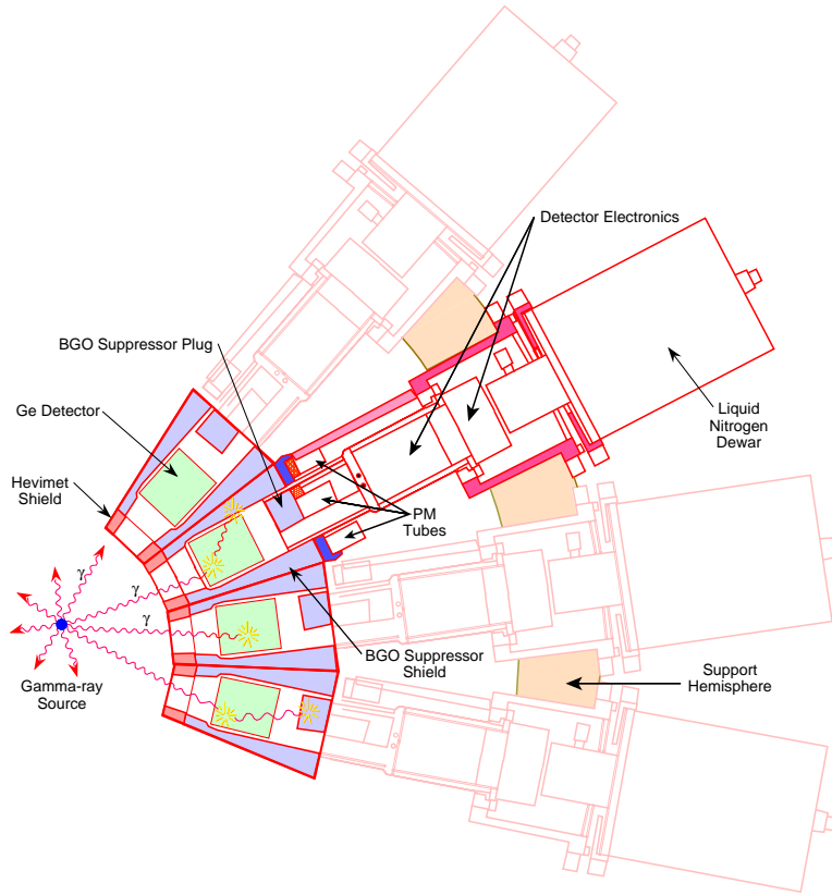
Figure 3-2: Diagram of the principal Gammasphere components [15]. The hevimet shields were not installed.
