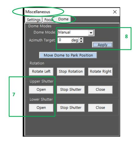
Figure 10: The **Dome** tab of **Telescope > Misc.**, by which one opens and closes the dome shutters, and sets the dome mode to track the telescope. Again: always open the upper shutter before the lower, and close it after the lower.
