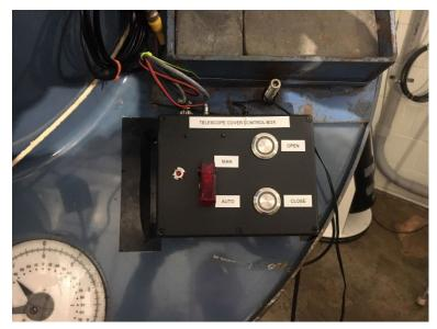
Figure 20: the telescope cover's manual override controls.
