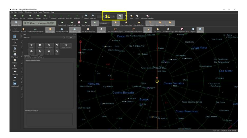
Figure 11: TheSky X just after startup. The **Connect** button has been pushed; the yellow circular target shows where the TCS thinks the telescope is pointed.
