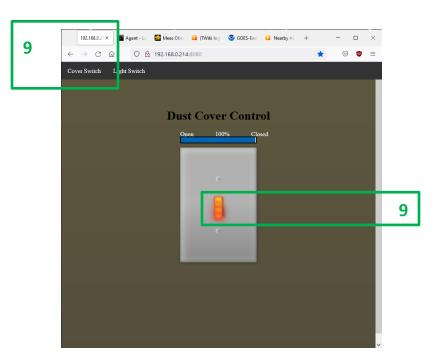
Figure 9: Firefox, with the telescope cover control (TCC, leftmost tab) in the foreground.
