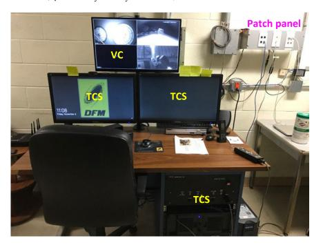
Figure 1: The Mees Observatory **telescope control system (TCS)** console, with its computer and three monitors. Uppermost is the video-camera (VC) monitor screen, which is connected to the DVR below and behind the right-hand TCS monitor. Also labelled is the patch panel at the end of data cables from the telescope and instruments.
