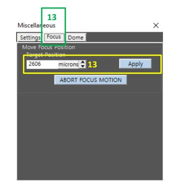
Figure 13: initializing the telescope focus. Note that the target position indicated in the figure is very far from the optimal focus for either of the CCD cameras; a star should look like a donut through the eyepiece in this setting.
