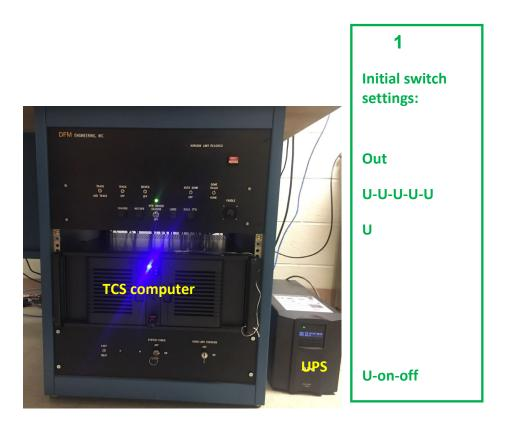
Figure 3: The Telescope Control System (TCS) front panel, and the settings that the switches should have when you enter the control room or start the system up from scratch (U = up, D = down).
