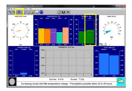
Figure 2: Current conditions at the Mees weather station, which is displayed by pushing the **Bulletin Window** banner button (indicated). Note the indoor and outdoor relative humidity values. The weather station itself is on top of the utility pole, across the driveway from the dome's loading dock.
