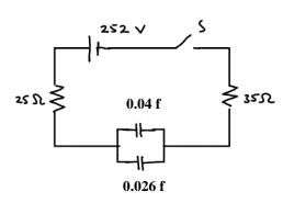
In the circuit to the left, how much energy is stored in the 0.026 farad capacitor 2 seconds after the switch S is closed?
