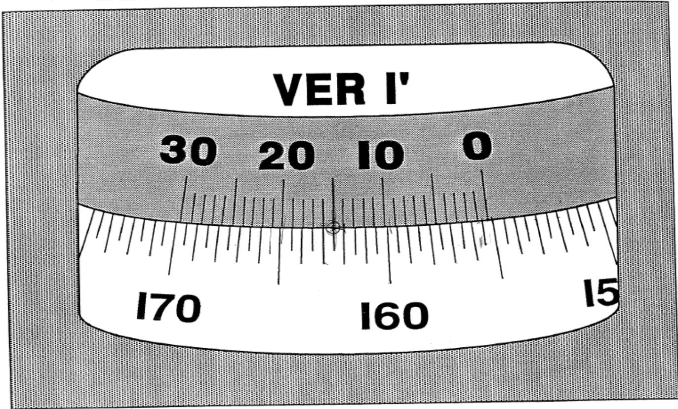
The relative rotational positions of the telescope base and the table base are measured using the vernier scales.
