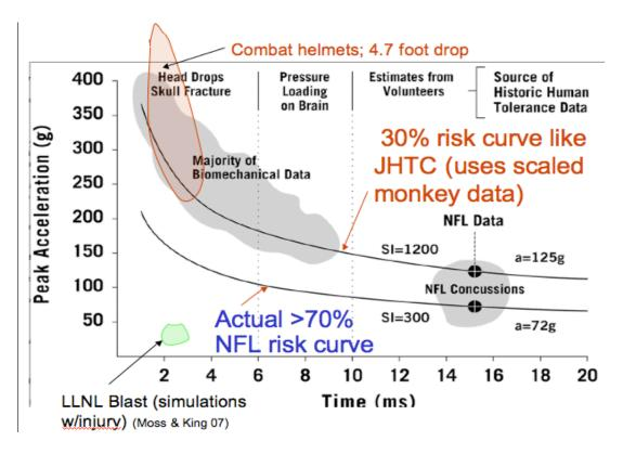
Figure 3.7: Comparison of current combat helmets, NFL football injuries, and blast injury on the acceleration vs. impact duration graph and the SI=300 and SI=1200 curves. Note that even by the JHTC standard, which is itself too weak (as exemplified clearly by NFL data) current combat helmets are ineffective.
