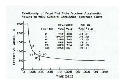
Figure 3.2: Wayne State Head Tolerance Curve (Patrcick 1963; Snyder 1970). Data are fit by the curve, which is extended well beyond the regime of the actual data.
