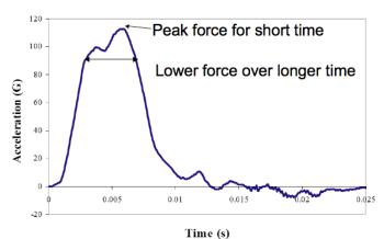
Figure 3.1: A typical time evolution curve for an acceleration (=magnitude of deceleration) of a helmeted headform subjected to a drop. The curve is meant for illustrative purposes but is roughly consistent with those from a 6kg head form with a currently used PASGT padded helmet system dropped from 3 feet. (e.g. Fig M-18 of Trimble et al. 05)
