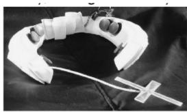
Figure 3.9: The Riddell VSR4 helmet with the 6, spring mounted accelerometers, battery pack, and antenna installed (Duma et al. 2005).
