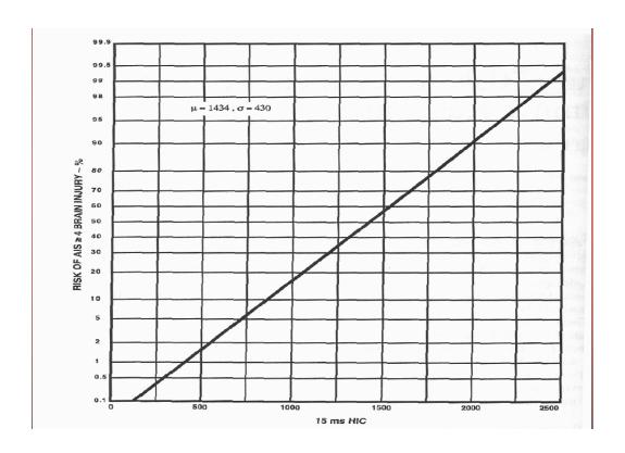
Figure 3.4: Typical injury risk curve associated with HIC. The vertical axis is the risk of injury and the horizontal axis is the HIC. The curve indicates the likelihood of concussion for a given HIC value (Prasad & Mertz 1985).
