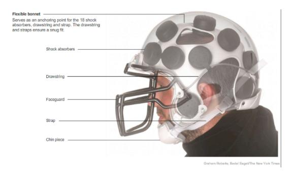
Figure 3.11: The Xenith X-1 helmet with the 18 air cushion shock absorbers described in the text (Schwarz 2007). This is a true paradigm shift in helmet design and is likely to make a substantial improvement in TBI protection from even the Ridell Revolution in Fig 3.11 as the design is refined.
