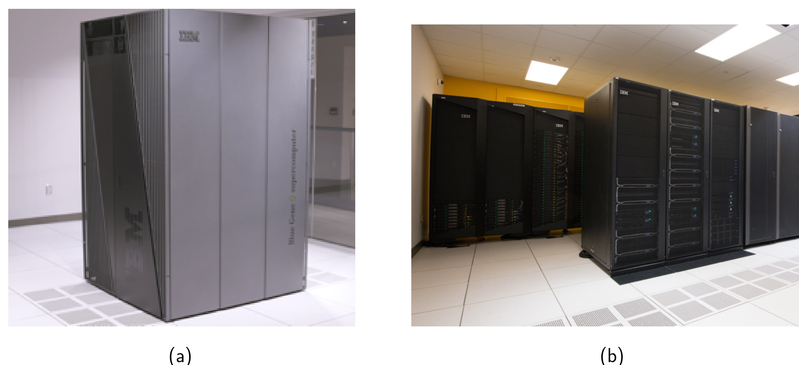
Figure 5: The Blue Gene/Q system and BlueHive Cluster at the University of Rochester: (a) BlueStreak(# 276 on the November 2014 Top500 list). It consists of 1,024 nodes, 16,384 CPU cores, 16 TB of RAM, and 400 TB of storage. (b) BlueHive. It consists of 284 nodes, 5,656 CPU cores, 21 TB of RAM. It includes the nodes with the Intel Ivy Bridge processors, NVIDIA's K20X GPUs and the Intel Phi 5110P accelerators.
