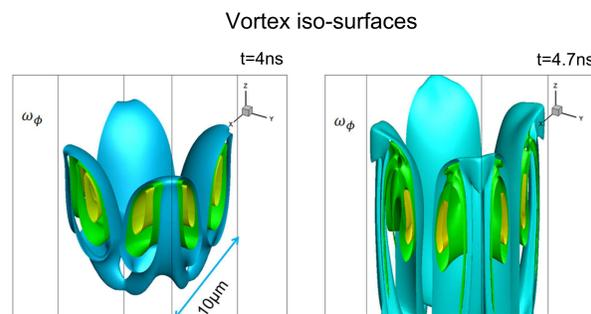
Figure 5: Azimuthal vortex  $\omega_\phi = \sqrt{\omega_x^2 + \omega_y^2}$  in the 3D bubble in an *ART3D* simulation. The distortion of the vortex enhances the bubble acceleration in 3D
