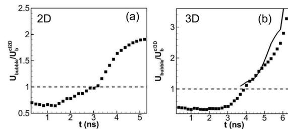
Figure 4: Ratio of the bubble velocities to the classical bubble velocities from the 2D (a) and 3D (b) ART simulations for the perturbation wavelength  $\lambda = 10\mu\text{m}$  (square). The solid line is given by  $U_b^{rot3D}$  in Fig. 6.
