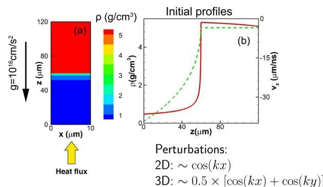
Figure 2: The simulation setup for the *ART3D* simulation with  $\lambda = 10\mu\text{m}$ . (a) The contour is the initial density profile. (b) The initial  $\rho$  (solid) and  $v_z$  (dashed) profiles along the  $z$  axis.
