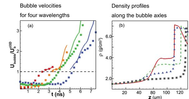
Figure 7: (a) The bubble velocities from *ART3D* (square) compared with  $U_b^{rot3D}$  (solid line) for  $\lambda = 40$ (red),  $20$ (orange),  $10$ (green),  $7$ (blue)  $\mu\text{m}$ , respectively. (b) The density profiles along the bubble axle. Solid:  $\lambda = 7\mu\text{m}$  at  $t = 6.8\text{ns}$ ; dashed:  $\lambda = 10\mu\text{m}$  at  $t = 5.7\text{ns}$ ; delta:  $\lambda = 20\mu\text{m}$  at  $t = 4.2\text{ns}$ ; square:  $\lambda = 40\mu\text{m}$  at  $t = 4.2\text{ns}$
