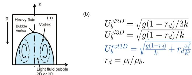
Figure 6: Theoretical model.  $U_b^{cl}$  are the asymptotic bubble velocities for classical (no ablation) RT.  $U_b^{rot3D}$  is the 3D bubble velocities with the vortex acceleration mechanism taken into account. The 2D version of this model has been verified in Ref. [1].
