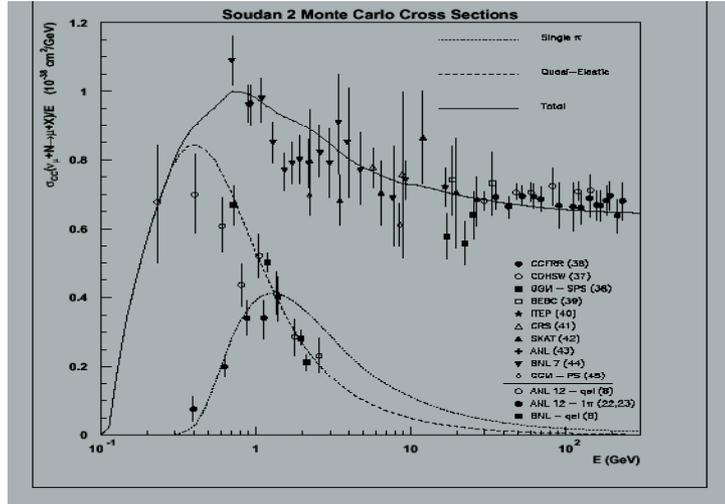
Figure 3: The total cross section for neutrinos as a function of energy with the single pion and quasi-elastic contributions shown.
