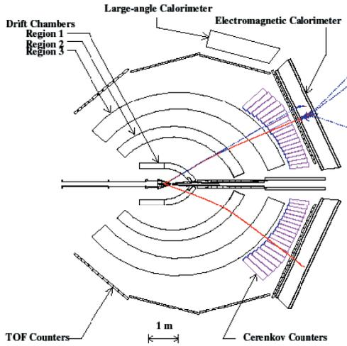
Figure 9: Side view of the CLAS detector, extracted from reference [33].
