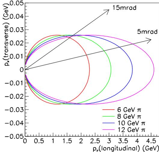
Figure 1: Schematic illustration of the off-axis beam technique. As can be seen, at a modest angle away from the focal axis of the pion beam (in this case, approximately  $1^\circ$  or 15 mr) pions of many different momenta all decay to neutrinos with approximately 1.5 GeV in an off-axis far detector.
