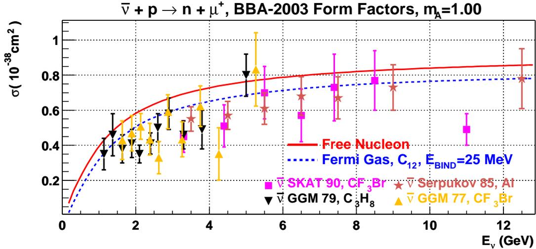
Figure 6: The QE antineutrino cross section along with data from various experiments. The solid curve uses no nuclear correction, while the dotted curve [22] uses a Fermi gas model for carbon with a 25 MeV binding energy and 220 MeV Fermi momentum. The data shown are from SKAT 1990 [27], GGM 1979 [32], Serpukov 1985 [30], and GGM 1977 [31].
