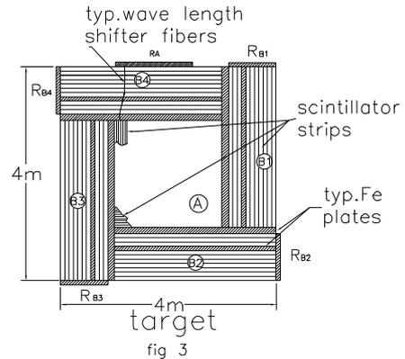
Figure 8: Concept of one plane of the active target in the near-source neutrino experiment.
