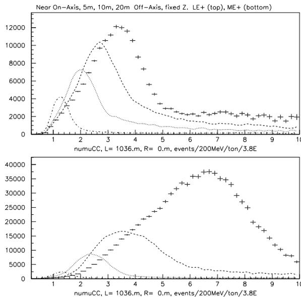
Figure 2: Relative event rate from the on and off-axis neutrino beams for the NuMI low energy (upper plot) and medium energy (lower plot) beams. The crosses correspond to the on-axis  $\nu_\mu$  neutrino-induced charge-current events, while the curves toward the left of the on-axis curve correspond to the event rates in detectors successively 5, 10, and 20 meters off axis, respectively.
