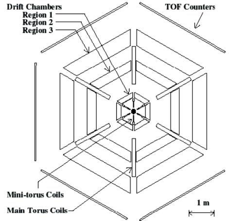
Figure 10: Beam view of the CLAS detector, extracted from reference [33].
