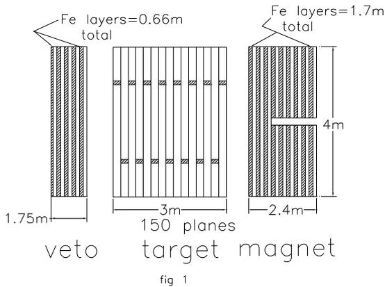
Figure 7: One concept of the near-source neutrino experiment planned for the NuMI beam at Fermilab, showing a 4 m x 4 m x 3 m active scintillator target, followed by a sampling calorimeter and magnetized range detector and preceded by an instrumented upstream veto.
