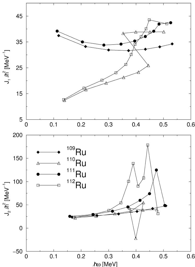
Fig. 5. The kinematical (top) and dynamical (bottom) moments of inertia as a function of the rotational frequency for the yrast states of <sup>109–112</sup>Ru.
