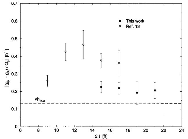
FIG. 5. Ratios of  $|(g_K - g_R)/Q_0|$  for the  $5/2^+[422]$  band in  $^{103}\text{Nb}$  are plotted as a function of spin. The dashed line is the value from the transitions of the  $\nu h_{11/2}$  band in  $^{105}\text{Mo}$  [22].
