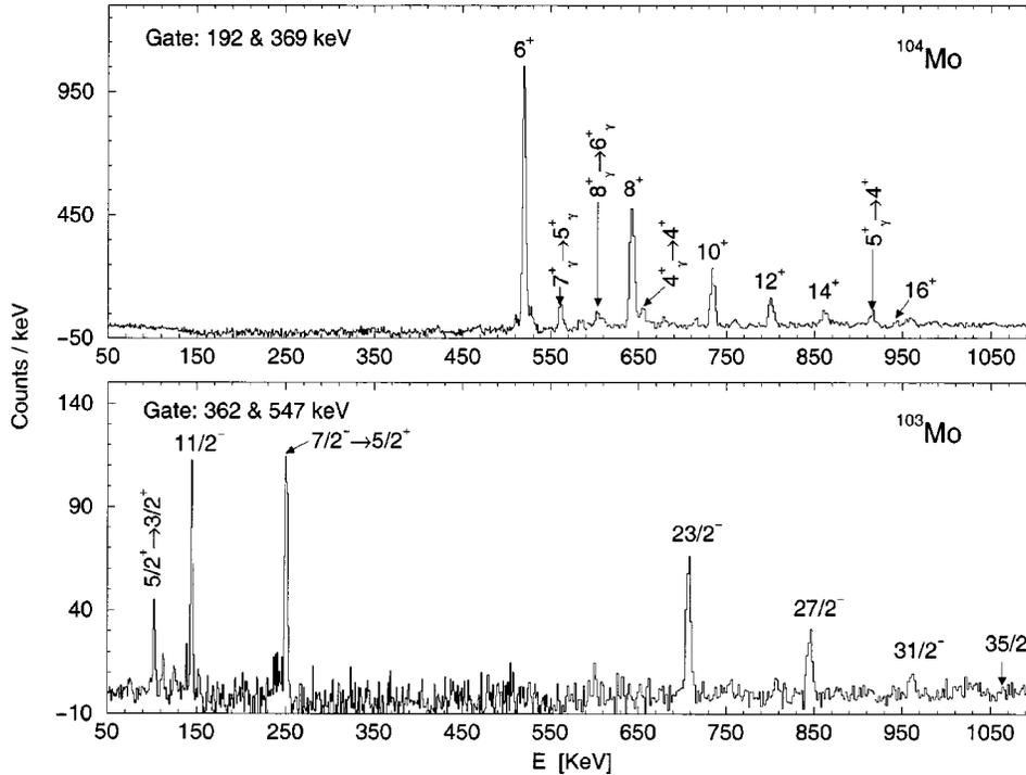
FIG. 1. Doppler-shift corrected spectra with gates on the mass and known  $\gamma$ -ray transitions in  $^{103}\text{Mo}$  (lower) and  $^{104}\text{Mo}$  (upper). The labeled transitions are  $\Delta I=2$  transitions unless specified otherwise explicitly. The uneven background observed in the upper spectrum for energy between 50 and 450 keV is due to the existence of broad  $\gamma$ -ray peaks from the partner nuclei, which have wrong Doppler-shift corrections.
