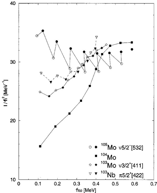
FIG. 4. The kinematical moment of inertia as a function of the rotational frequency for the  $3/2^+[411]$  band in  $^{103}\text{Mo}$ ,  $5/2^- [532]$  band in  $^{105}\text{Mo}$ , ground-state band in  $^{104}\text{Mo}$ , and  $5/2^+[422]$  band in  $^{103}\text{Nb}$ . The convention used in calculating the moment of inertia and rotational frequency is from Ref. [24].
