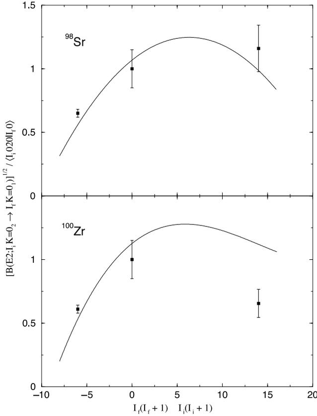
FIG. 2. The Mikhailov plot for the interband transitions between the second  $2^+$  state and members of the ground-state band. The solid lines are the best fits to the data according to Eq. (5) with the  $M_2/M_1$  ratio fixed to  $-0.058$  and  $-0.067$  for  $^{98}\text{Sr}$  and  $^{100}\text{Zr}$ , respectively.
