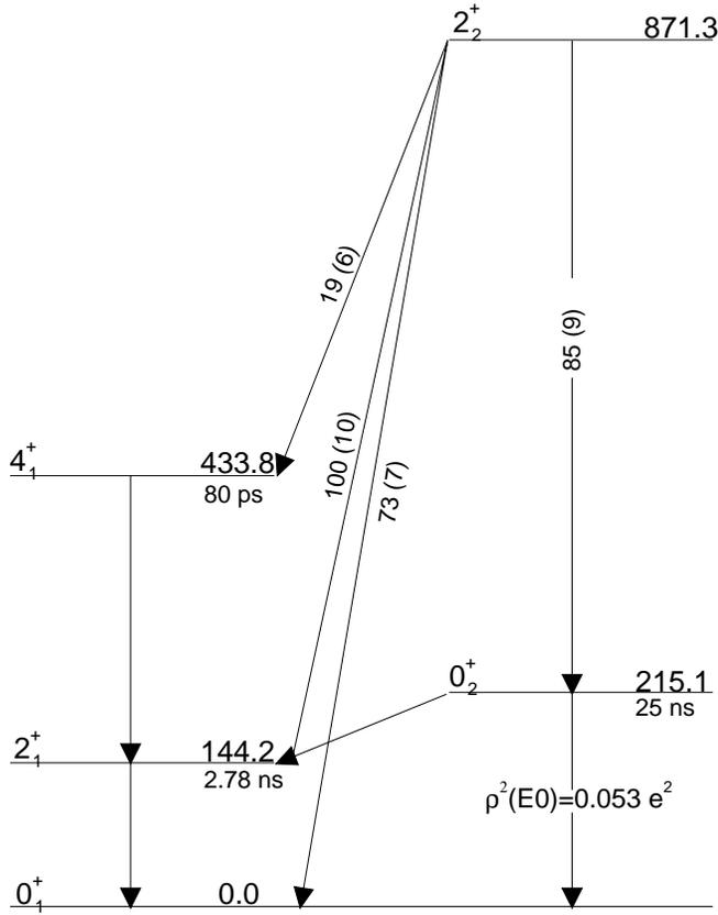
FIG. 1. Partial level scheme of <sup>98</sup>Sr. Energies are in keV. The known half-lives and  $\gamma$ -ray branching ratios for the second 2<sup>+</sup> decay also are listed. The 2<sub>2</sub><sup>+</sup> → 2<sub>1</sub><sup>+</sup> transition is assumed to be pure E2 in the calculations.
