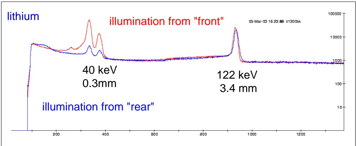
No measurable resolution difference between front and back illumination.....suggests not bulk trapping
