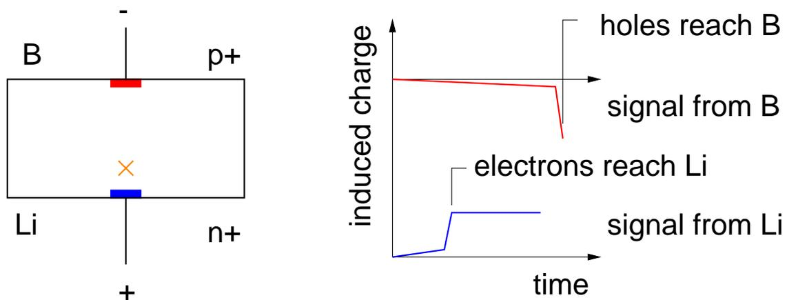
Single-polarity charge sensing:
