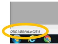
Figure 16: cursor readout at lower left in CCDSoft's main window, showing pixel coordinates X and Y, measured from upper left, and the value of the signal in this pixel, in DN.
