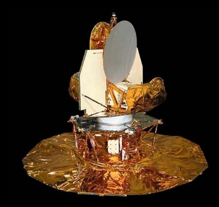
The NASA Wilkinson Microwave Anisotropy Probe (<u>WMAP</u>), launched in 2001, which obtained definitive images of cosmic background fluctuations.
