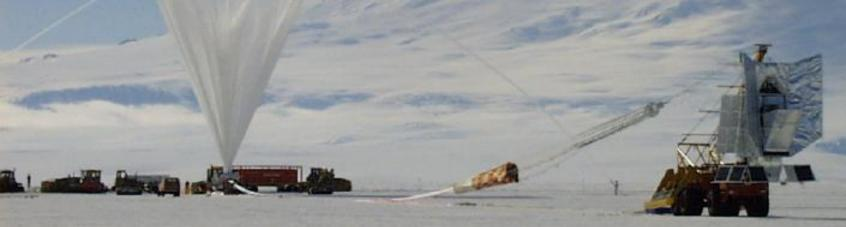
Deployment of the balloon-borne **BOOMERANG** cosmic-background anisotropy experiment in Antarctica; Mt. Erebus in the background.
