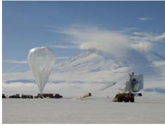
Image: Deployment of the balloon-borne BOOMERANG cosmic-background anisotropy experiment in Antarctica, with Mt. Erebus in the distance (Caltech/UCSB/U. Rome/NASA).
