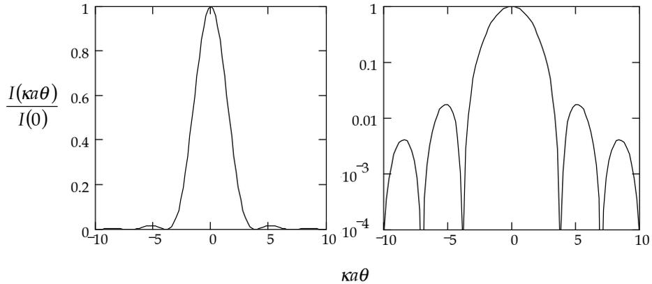
Figure 13.3: plots of the intensity given by Equation 13.15, on linear (left) and logarithmic (right) scales.
