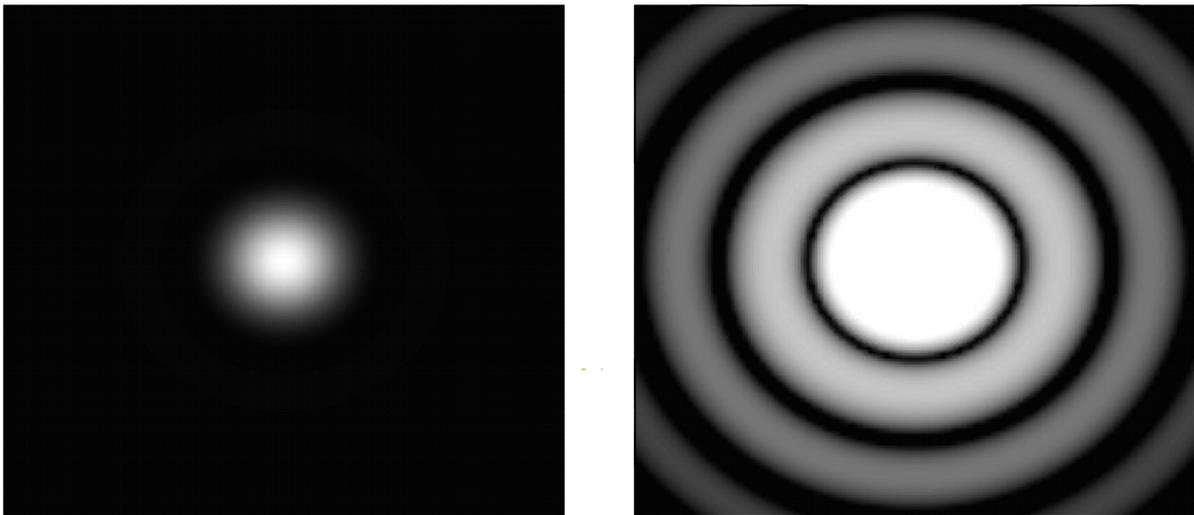
Figure 13.4: grayscale images of the far-field intensity diffracted by a circular aperture. Left: linear scale, for emphasis of the structure of the central maximum. Right: logarithmic scale with the central maximum “saturated” for intensity greater than  $10^{-1.3}$  of the peak value, for emphasis of the surrounding bright and dark rings. Figure 13.3 consists of meridional cross sections of these images.
