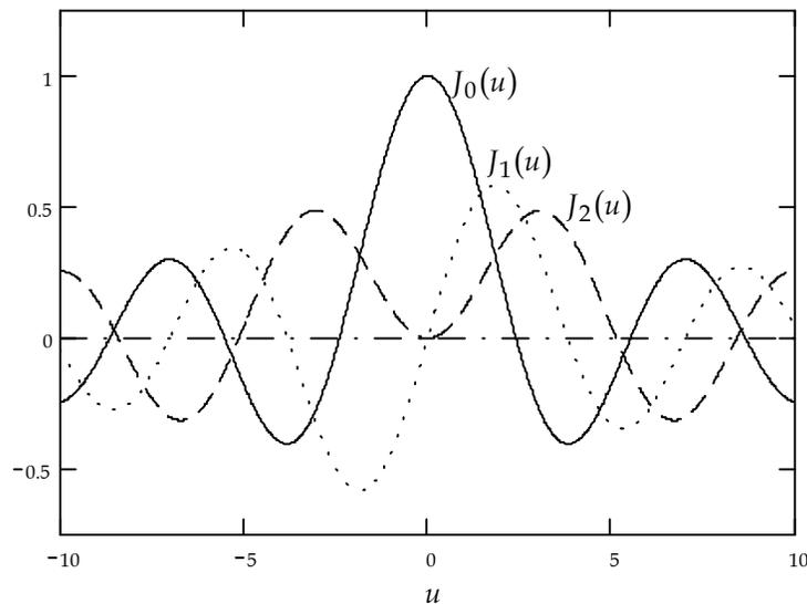
Figure 13.2: The first three of the first-kind Bessel functions.
