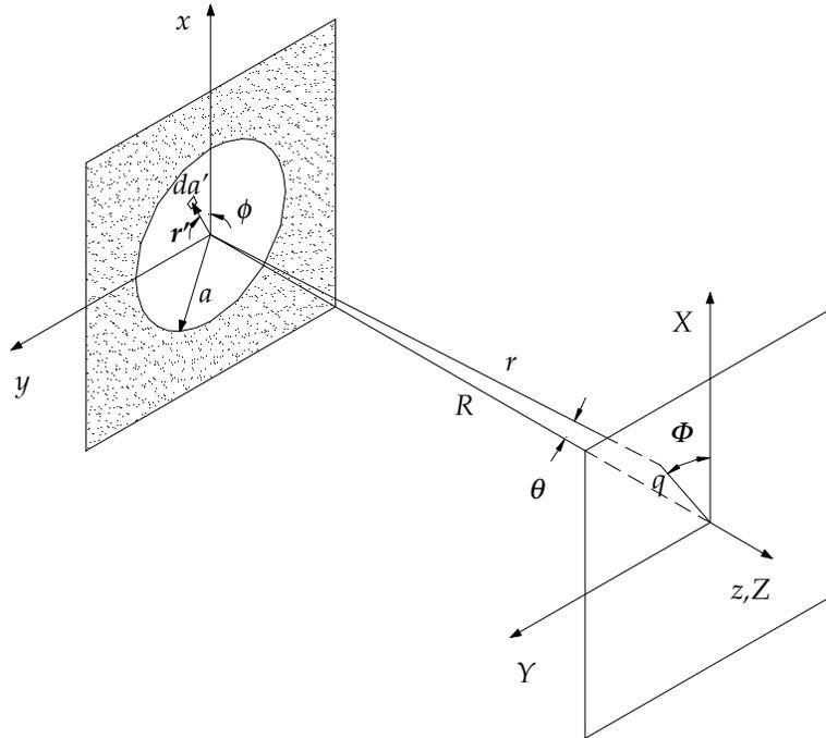
Figure 13.1: geometry of circular aperture and distant screen for calculation of diffraction of plane wave incident normally on the aperture. The “screen” axes  $X$  and  $Y$  are parallel to the “aperture” axes  $x$  and  $y$ .
