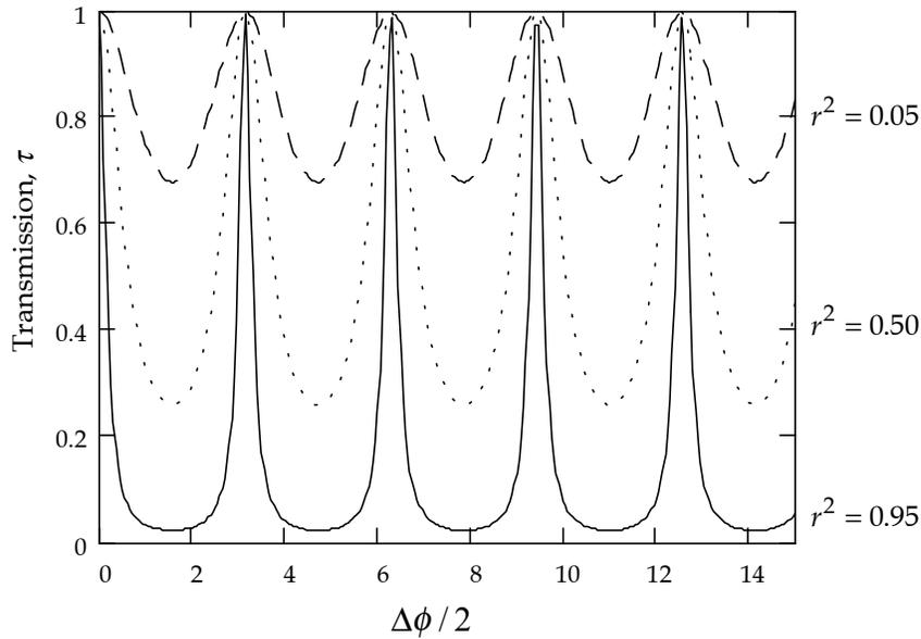
Figure 26.1: the Airy function, the transmission of the Fabry-Perot interferometer.
