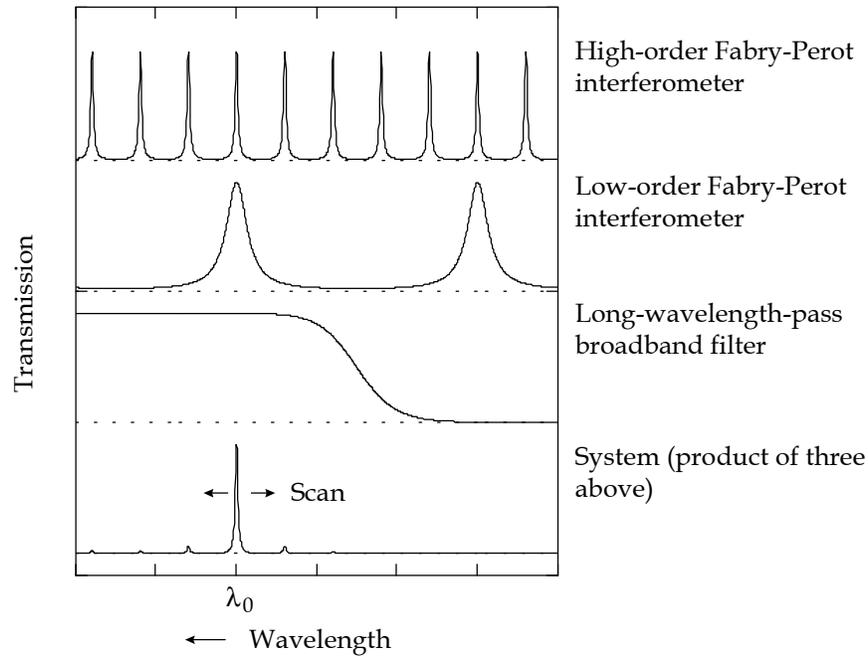
Figure 26.2: Transmission of a tandem Fabry-Perot spectrometer.
