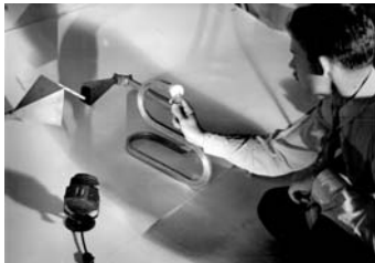
Malcom Strandberg (MIT) demonstrates collection and transmission through serpentine waveguide of microwave power large enough to light up the neon bulb he’s holding. (Fritz Goro, Life Magazine photo, 1945.)
