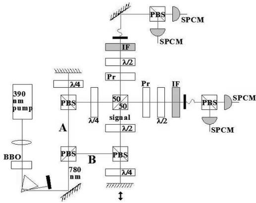
FIG. 2: Schematic of the experimental setup. The downconverted photons are separated at the first PBS. The photon from arm A is circularly polarized when it is incident on the 50/50 BS. HOM interference occurs when the path lengths of arms A and B are matched, leading to cloning of the linearly polarized photon from arm B after post-selection.
