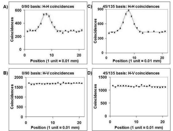
FIG. 3: The figures show the results of measuring same port coincidences with respect to path length mismatch for the four possible polarization combinations. The *position* axes are only for scale, and have a systematic offset of  $\sim 0.08$  mm. Boson mode enhancement only occurs in A and C where both photons have the same polarizations, thus leading to the cloning effect.
