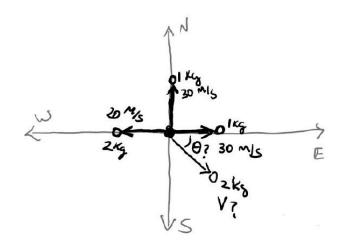
fragment moves west at 20 m/s. Unfortunately the proving ground technicians failed to record the direction and speed of the fourth fragment, though they were able to determine its mass as 2 kg. To satisfy your curiosity and to exercise your amazing dexterity in physics, you determine the direction and speed of the fourth fragment ... (please do/repeat that calculation below). You might find it useful to know the trig identitity  $(\sin\theta)^2 + (\cos\theta)^2 = 1$ .
