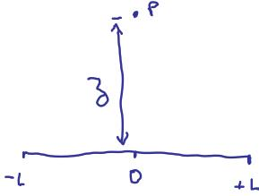
Find É at a point p a distance 3 above the Midpoint of a line segment of length 21. Which carries a uniform line charge of  $\lambda$ .
