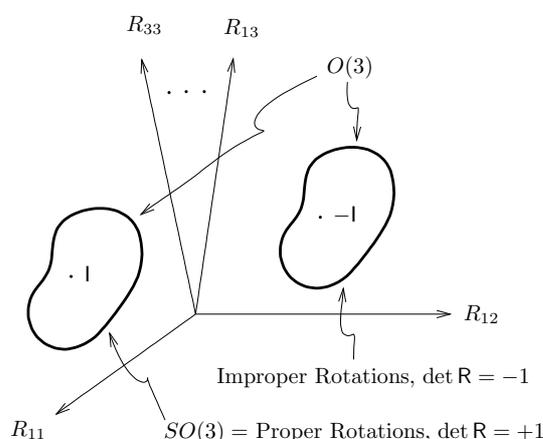
**Fig. 3.** The rotation group  $O(3)$  can be thought of as a 3-dimensional surface imbedded in the 9-dimensional space of all  $3 \times 3$  matrices. It consists of two disconnected pieces, one of which contains the proper rotations and constitutes the group  $SO(3)$ , and the other of which contains the improper rotations. The proper rotations include the identity matrix  $I$ , and the improper rotations include the parity matrix  $-I$ .
