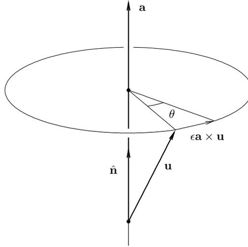
**Fig. 1.** The axis  $\hat{\mathbf{n}}$  of a near-identity rotation matrix  $\mathbf{R} = \mathbf{I} + \epsilon \mathbf{A}$  is in the direction of the vector  $\mathbf{a}$  associated with the antisymmetric matrix  $\mathbf{A}$ . The small angle of rotation is  $\theta = \epsilon |\mathbf{a}|$ .
