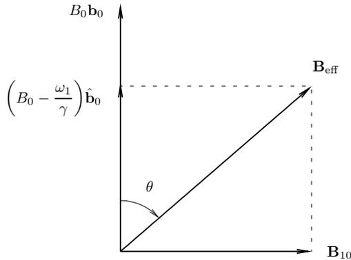
**Fig. 3.** In the rotating frame, the field  $\mathbf{B}_1 = \mathbf{B}_{10}$  is stationary, and  $\mathbf{B}_0$  is reduced in magnitude by  $\omega_1/\gamma$ . The resulting field is  $\mathbf{B}_{\text{eff}}$ , which is constant in the rotating frame.
