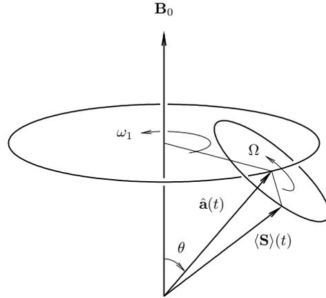
**Fig. 4.** The expectation value of the spin  $\mathbf{S}$  precesses about the axis  $\hat{\mathbf{a}}(t)$  with frequency  $\Omega$ , while that axis itself precesses about  $\mathbf{B}_0$  with frequency  $\omega_1$ .
