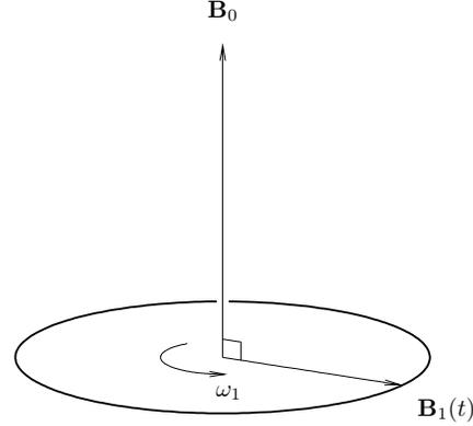
**Fig. 2.** The field in magnetic resonance experiments consists of a constant field  $\mathbf{B}_0$  plus a time-dependent field  $\mathbf{B}_1(t)$  that is perpendicular to  $\mathbf{B}_0$  and that rotates about  $\mathbf{B}_0$  at frequency  $\omega_1$ .
