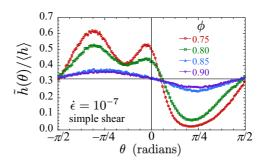
FIG. 14. Average force-moment per radian  $\tilde{h}(\theta)$ , normalized by the average force moment  $\langle h \rangle$ , in simple shearing. Results are plotted vs bond angle  $\theta$  for several different packing fractions  $\phi$  at strain rate  $\dot{\epsilon} = 10^{-7}$ . The solid horizontal black line at  $\tilde{h}/\langle h \rangle = 1/\pi$  represents the average value. The system has N = 32768 particles.
