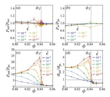
FIG. 4. Stress ratios comparing uniaxial compression, isotropic compression, pure shear, and simple shear. Pressure ratios (a)  $p_{\rm uni}/p_{\rm iso}$ , (b)  $p_{\rm ss}/p_{\rm ps}$ , (c)  $p_{\rm uni}/p_{\rm ps}$ , and (d) shear stress ratio  $\sigma_{\rm uni}/\sigma_{\rm ps}$  vs  $\phi$  for different strain rates  $\dot{\epsilon}$ . The vertical dashed line indicates the isotropic compression-driven jamming  $\phi_J = 0.8415$ . The system has N = 32768 particles.
