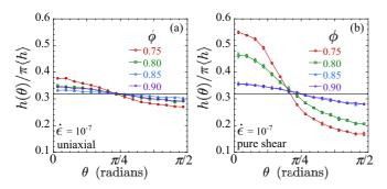
FIG. 8. Average force-moment on a contact bond at angle  $\theta$ ,  $h(\theta) = \tilde{h}(\theta)/\mathcal{P}(\theta)$ , normalized by  $\pi \langle h \rangle$ , vs  $\theta$  for several different packing fractions  $\phi$  at strain rate  $\dot{\epsilon} = 10^{-7}$ . Panel (a) is for uniaxial compression, while panel (b) is for pure shearing. The solid horizontal black line at  $\tilde{h}/\pi \langle h \rangle = 1/\pi$  represents the average value. The system has  $N = 32\,768$  particles.
