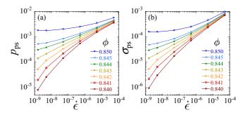
FIG. 24. (a) Pressure p and (b) shear stress  $\sigma$  vs strain rate  $\dot{\epsilon}$ , in steady-state pure shearing, for several different values of packing  $\phi$  near jamming. The system has N = 32768 particles.
