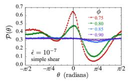
FIG. 13. Probability density  $\mathcal{P}(\theta)$  for the contact network to have a bond directed at angle  $\theta$  with respect to the flow direction  $\hat{\mathbf{x}}$ , in simple shearing. Results are plotted vs  $\theta$  for several different packing fractions  $\phi$  at strain rate  $\dot{\epsilon} = 10^{-7}$ . The solid horizontal black line at  $\mathcal{P} = 1/\pi$  represents the average value. The system has N = 32768particles.
