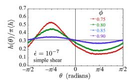
FIG. 15. Average force-moment  $h(\theta) = \tilde{h}(\theta)/\mathcal{P}(\theta)$ , normalized by  $\pi \langle h \rangle$ , in simple shearing. Results are plotted vs bond angle  $\theta$ for several different packing fractions  $\phi$  at strain rate  $\dot{\epsilon} = 10^{-7}$ . The solid horizontal black line at  $\tilde{h}/\pi \langle h \rangle = 1/\pi$  represents the average value. The system has N = 32768 particles.
