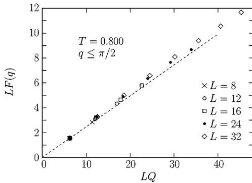
FIG. 3. Scaling collapse of  $LF(q)$  vs  $LQ$  at  $T_c$ , for  $L = 8-32$ ,  $q < \pi/2$ .  $LF(q)$  vanishes linearly as  $LQ \rightarrow 0$ .
