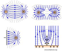
In this figure, the thick blue lines are the electric field lines. The dashed lines are the equipotential surfaces.
