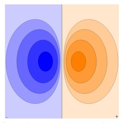
Shown above ( is a cross-section) of the equipotential surfaces of a dipole oriented along the horizontal axis.
