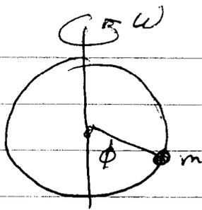
$$T = \frac{1}{2} m v^2 = \frac{1}{2} m (R^2 \dot{\phi}^2 + R^2 \sin^2 \phi \omega^2)$$
