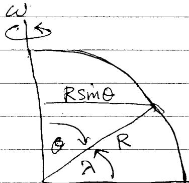
$$\begin{aligned}|\vec{\omega} \times (\vec{\omega} \times \vec{R})| &= \omega^2 R \sin \theta \\ &= \omega^2 R \cos \lambda\end{aligned}$$
