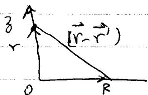
$$\vec{B}(z) = \int_0^{2\pi} d\phi \frac{R}{c} I \hat{\phi} \times \frac{[-R \hat{r} + z \hat{z}]}{(z^2 + R^2)^{3/2}}$$
