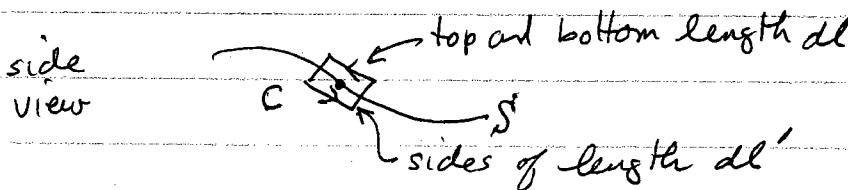
$$\nabla \times \vec{E} = 0 \Rightarrow \oint_C d\vec{l} \cdot \vec{E} \quad \text{since } \vec{E} \text{ is finite at surface,}$$
