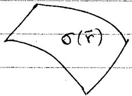
← a general surface  $S$  with surface charge density  $\sigma(\vec{r})$  for  $\vec{r}$  on  $S$ .  $\sigma(\vec{r})da$  is total charge in area  $da$  on surface
