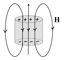
The top surface with  $\sigma_M = +M$  acts as source for **H** field lines, while the bottom surface with  $\sigma_M = -M$  acts as a sink for **H** field lines.
