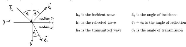
We know that  $\omega_0 = \omega_1 = \omega_2 \equiv \omega$ , and that  $k_{0x} = k_{1x} = k_{2x}$  (the  $k_y$  components for each wave vanish).
