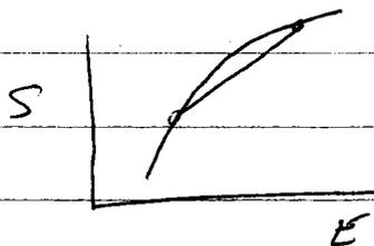
concave  $\equiv$  the cord drawn between any two points on curve lies below the curve
