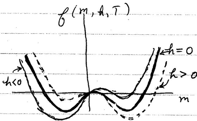
as  $h$  goes smoothly through zero, the value of  $m$  that minimizes  $f(m, h, T)$  jumps discontinuously from  $+m_0$  to  $-m_0$ .
