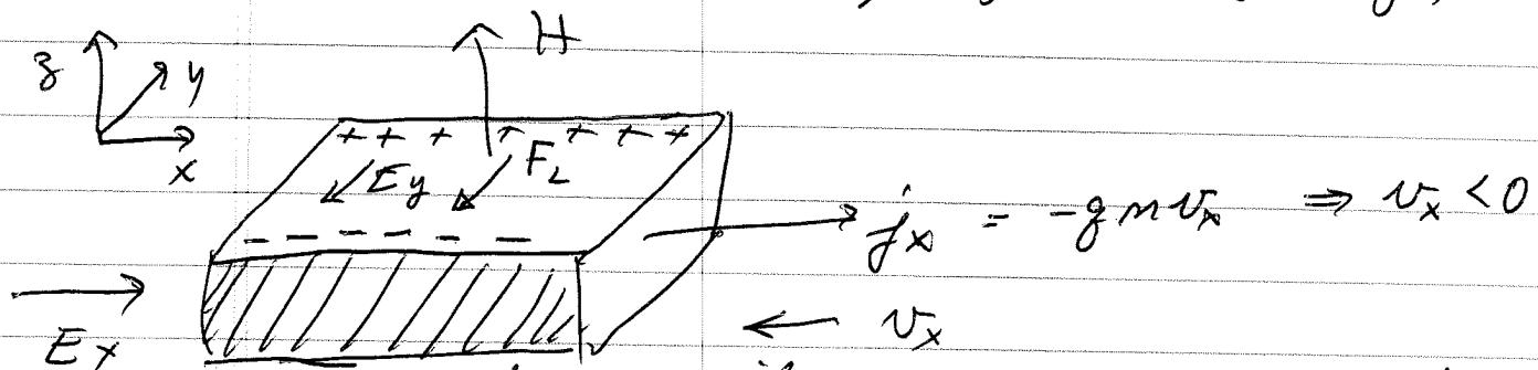
$F_L$  deflects the mobile negative charges carrying the current, and negative charges build up on shaded surface
