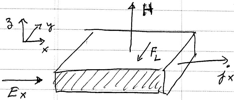
Electric field  $E_x$  applied in  $\hat{x}$  direction produces flowing electric current  $j_x$  in  $\hat{x}$  direction. Magnetic field  $H$  in  $\hat{z}$  direction exerts
