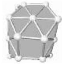
Fig. 2.9: A hexagonal prism gold nanocluster with 30 atoms. Courtesy of Wilson and Johnston from Ref. [46].
