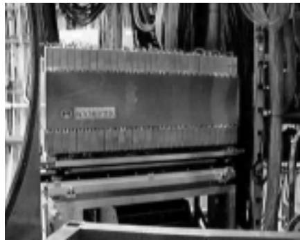
One of the PHOBOS time-of-flight sections installed at RHIC, replete with the Rochester seal
