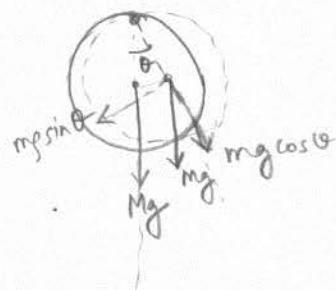
$T = 2.0 \text{ s}$   $R = ?$  (radius of hoop),  $m = \text{mass of hoop}$  (not given)
