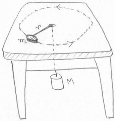
A dice of mass  $m$  slides on a frictionless table while attached to a hanging cylinder of mass  $M$  by a cord through a hole in the table. What speed keeps the cylinder at rest?
