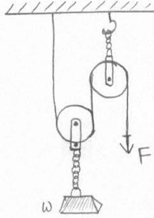
On this figure, a worker lifts a weight  $w$  by pulling down on a rope with a force  $\vec{F}$ . The upper pulley is attached to the ceiling by a chain, and the lower pulley is attached to the weight by another chain. In terms of  $w$  find the tension in each chain and the magnitude of  $\vec{F}$  if the weight is lifted at constant speed. Include all free body diagrams in the answer. Assume that the rope, pulleys and chains all have negligible weights.
