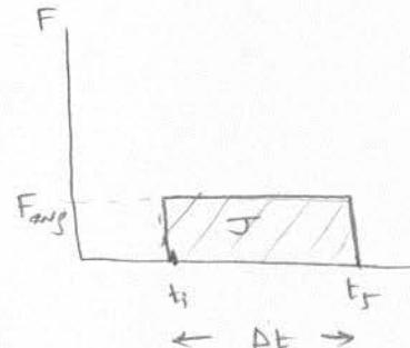
$$\vec{P}_f - \vec{P}_i = \Delta \vec{p} = \int_{t_i}^{t_f} \vec{F} dt = \vec{J}$$
