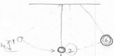
$$v_{1f} = \frac{m_1 - m_2}{m_1 + m_2} v_{1i} = \frac{0.030 - 0.075}{0.030 + 0.075} (1.252 \text{ m/s}) = -0.537 \text{ m/s}$$
