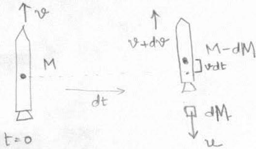
Note: The CM continues to move with the same initial velocity  $v$  but the rocket (of new mass  $M-dM$ ) moves with velocity  $(v+dv)$  after  $dt$  time
