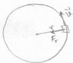
$$F_{fr} = \frac{mv^2}{r} = F_{\text{applied}} \quad N = mg$$
