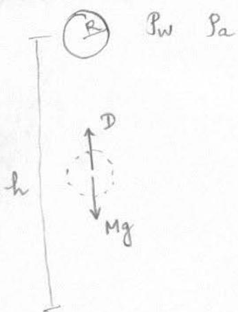
To reach terminal speed the drag force must completely balance the weight of the drop.
