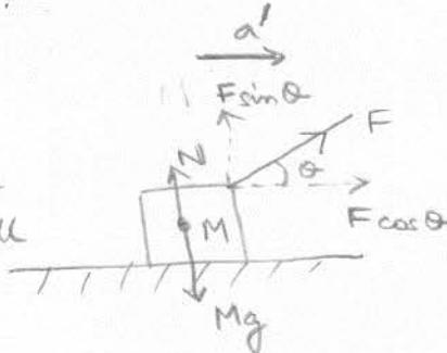
$$\left. \begin{array}{l} F \cos \theta - \mu N = Ma \\ Mg + F \sin \theta = N \end{array} \right\}$$
