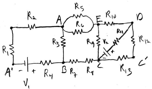
For this, I'm using step 0; reduce using addition rules for resistors!
