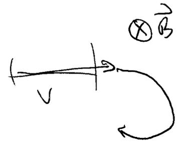
$$\vec{F}_{\text{mag}} = q \vec{v} \times \vec{B} \quad \sin \theta = \sin 90^\circ = 1$$
