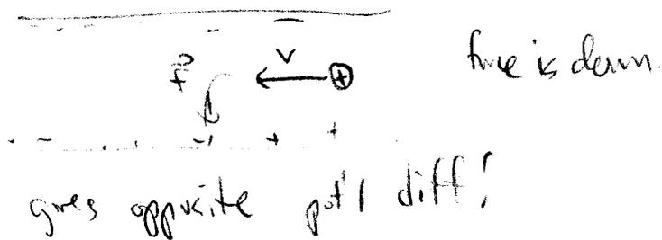
→ this first revealed that it is neg charges moving inside conductors
