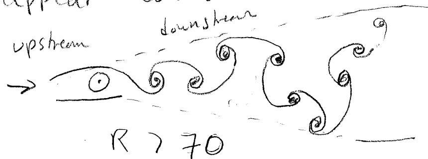
The vortices appear in a "wake" that increases in width farther downstream, (= "Karman vortex sheet")
