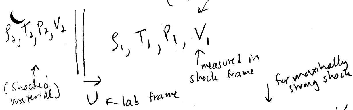
$$\text{For gas with } \gamma = \frac{5}{3}, \quad \frac{S_2}{S_1} = 4, \quad \frac{V_2}{V_1} = \frac{1}{4}$$
