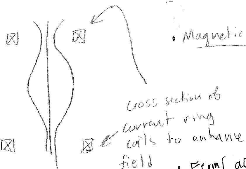
• Magnetic Bottle - can be used to trap and confine particles in Laboratory Devices.
