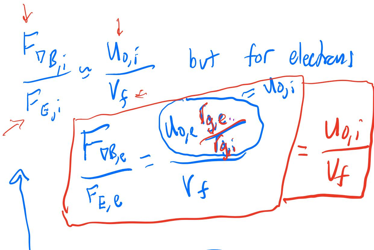
$$F_{\text{drift}, \nabla B, e} \approx \frac{e U_{0,e}}{c} r_{g,e} \frac{B}{r_{g,i}}$$
