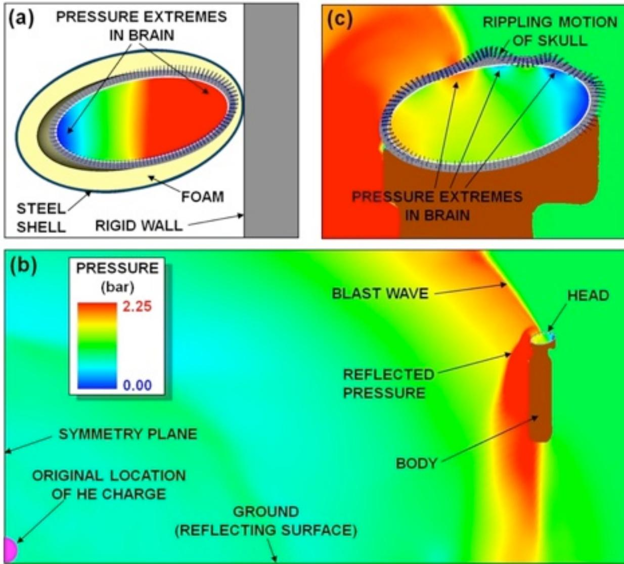
Blast wave at 5.6 ms after detonation
