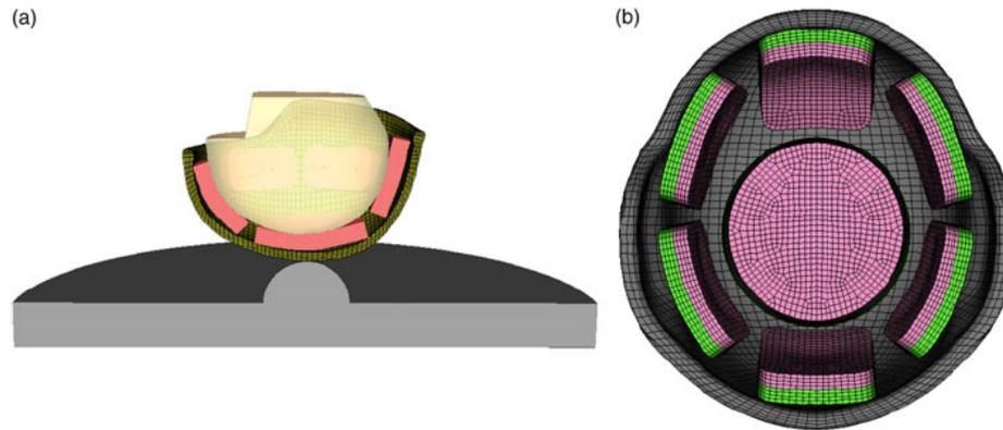
Figure 3. Geometry used to simulate USAARL experiment shown in Figure 2. (a) The half-model that was used for the simulations consists of 60,000 elements. Zoning in the helmet is shown. The headform is transparent in order to view the side pads. (b) Interior view of the complete helmet and pads.
