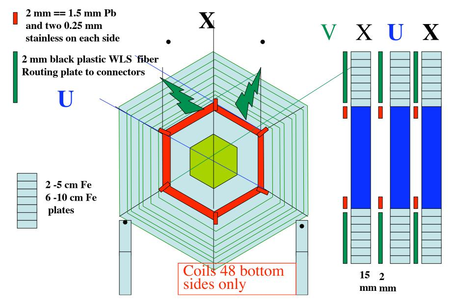
20 planes of HAD calorimeter downstream to fit within 4.4 m tunnel.
