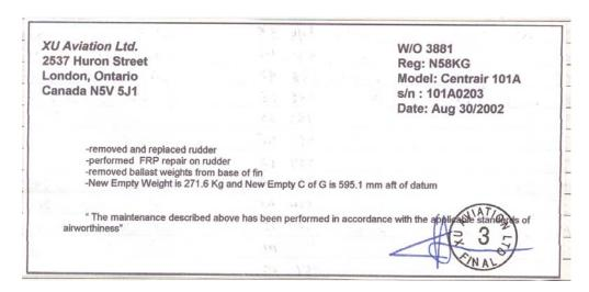
The 8/30/2004 weight and balance for Pegasus 101A0203 lists a new empty weight of 271.6 Kg and empty C of G at 0.5951m. Using this information gives the following load restrictions for the equipped pilot, i.e. pilot plus parachute plus drinking water etc.
