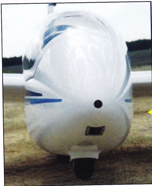
Note the centre tow-hook location and the re-positioned tailplane
