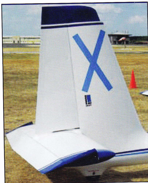
Note the centre tow-hook location and the re-positioned tailplane
